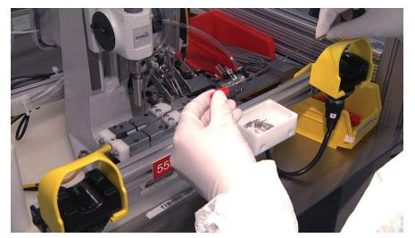
A Conmed employee assembles components for an electrosurgical device.
